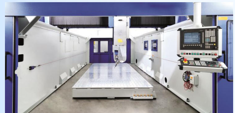
G-S-F/M Milling system in Gantry construction for special modelling
