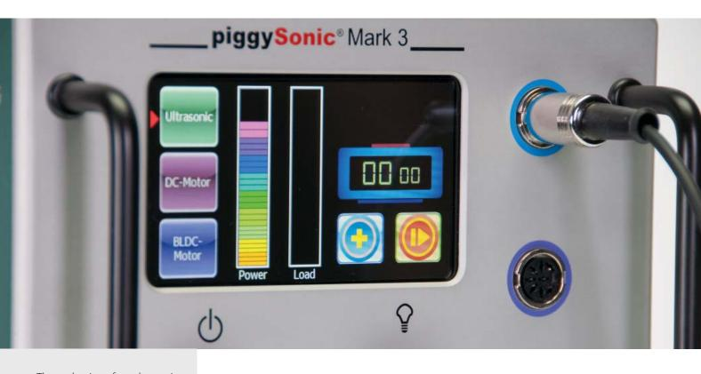
The selection for ultrasonic can be seen on this display. The output has already been defined. The start button has not yet been pressed, which is why nothing is displayed yet in the load diagram and the chronometer is not yet running.
