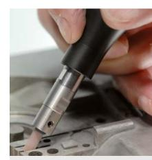
Have you ever experienced the problem when the ceramic-fibre file does not work as it should? The cause of this problem lies in the point-type clamping of conventional holders.
