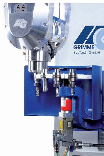
Tool change magazine 12/24 positions tool length up to 260 mm
