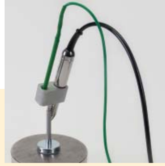
Holding device for hand piece with strong magnet
