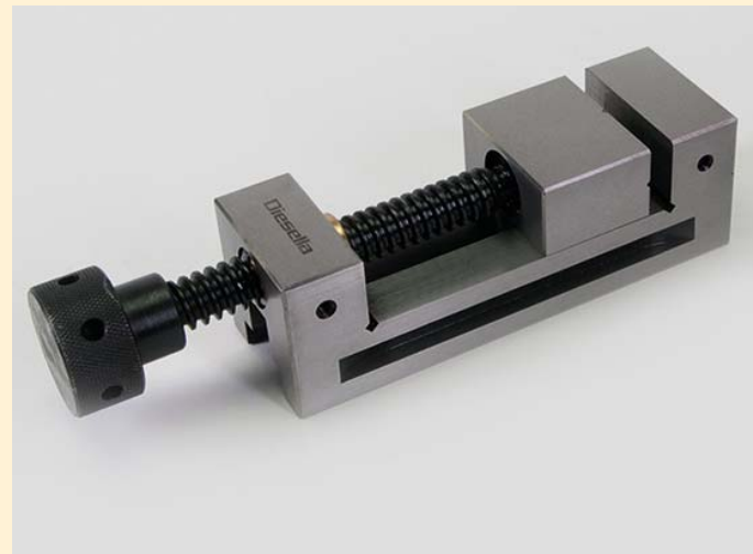
Vice Made of high-quality steel (20CrMnTi), hardened on 58 - 62 HRC with a parallelism of \pm 5 \mu\text{m} .
