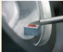
easyLap is very well suited for processing of smaller surfaces of a large 3D contour.
